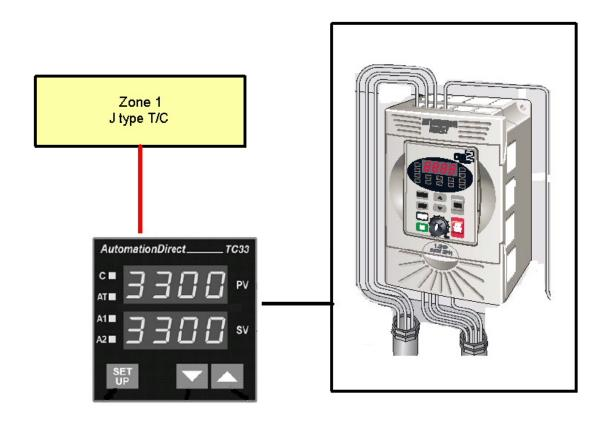
4-20 ma analog signal to GS2 drive controlling cooling blower to single zone furnace.
