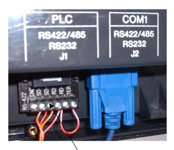
The RS485 SG+ and SG- come into top terminal for breakout.
