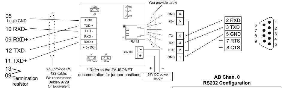
**Note:** The Termination resistor is built in to the panel.
