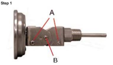
Loosen but do not remove the two- clamp retaining screws labeled "A" and the angle adjustment screw labeled "B".
