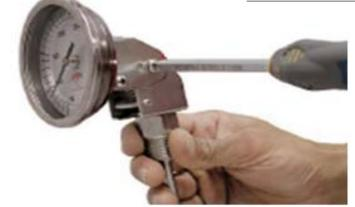
Rotate the clamp and adjust the angle of the dial face to the desired position and tighten all of the screws to secure.
