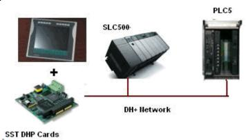
3.2) STRIO: This driver implements the AB Remote I/O protocol Scanner Mode to the family PLC5 using the SST
