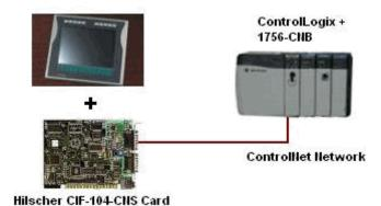
**2.2) DEVN:** This driver implements the **DeviceNet** slave using **Hilscher SMS-CIF104-DNS** PC card. This card has its firmware compiled also for WinCE and it has in the PC-104 format. So, in this case, you would need to install the Hilscher card CIF-104-DNS on your WinCE panel and this is will be a slave in the DeviceNet Network.
