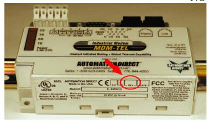
3. You can also detect the modem type using HyperTerminal. Please see the last section of this technical note for pointers on how to configure HyperTerminal to send AT commands to modem. To query the firmware version enter the **ati3<enter>**. Please see the tables below for information on how to interpret this firmware rev number.
