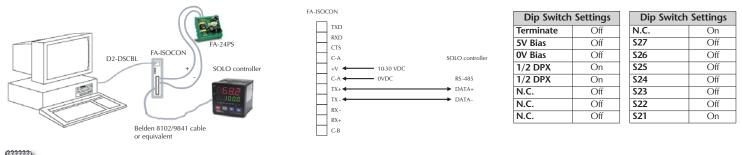
Note: In the configuration shown above, if the PC serial port is not available but a USB port is available, use the USB-RS232 (USB to RS232 converter cable) between the PC and the D2-DSCBL.
