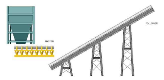
Both conveyors are engineered to move the same amount of material when in sync. The mechanical part of this example project will not be discussed in this document.
