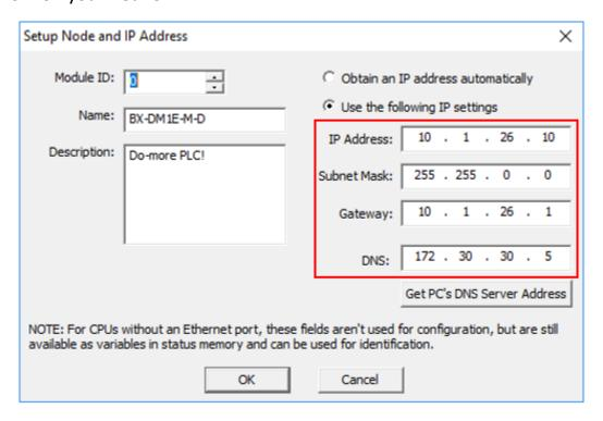
Probably one of the most common mistakes made when setting up Do-More to send email (or to be accessible on the Internet) is not specifying the Gateway address. The Do-More CPU cannot respond to nor target an IP address that is not on its subnet without the Gateway (which a public IP address WILL be). The default gateway IP address is the IP address of the router.
