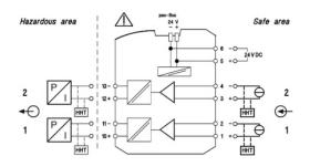
The Isolating Repeater Output is an associated apparatus as well as a nonincendive apparatus for installation in SAFE AREA and provides intrinsically safe circuits for field devices located in HAZARDOUS AREAS.
