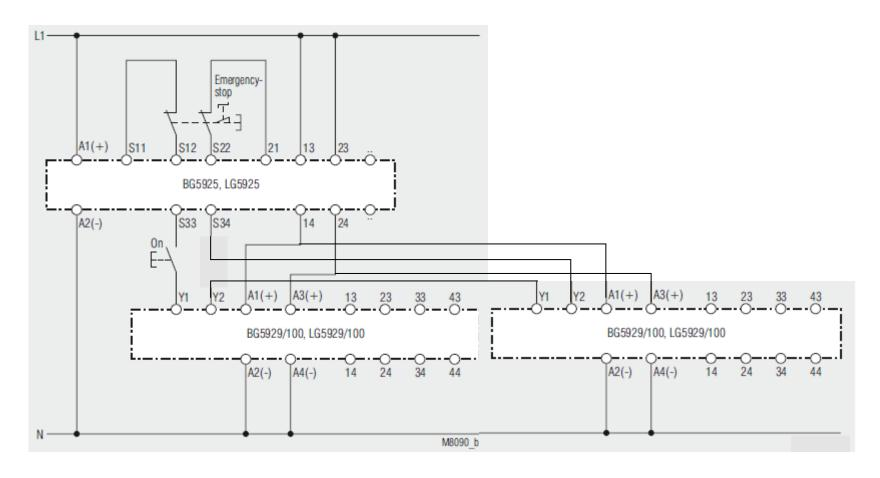
To add more extension modules connect the control inputs A1 and A3 in parallel, A2 and A4 to N or Ground, connect Y1 and Y2 in series into the start loop.
