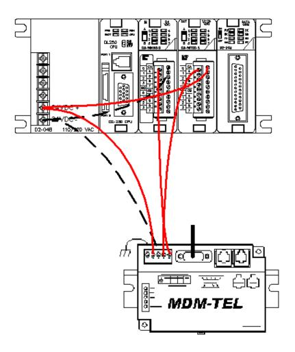
You must make sure that you use the correct I/O cards for this. The output from the PLC to initiate the dialing of the PLC requires either a relay output card or a DC sourcing card. The output from the MDM requires a sourcing input. Some examples are:
