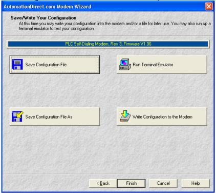
7. The modem is now configured for use. Depending on your intended function you may possible need to configure a Windows Modem Driver, DirectSoft New Link using the Modem Driver, KEPDirect New Channel using the Modem Driver, or PLC Rung Logic which uses the modem.
