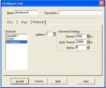
5. Choose Accept when complete and click "Yes" to check the connection. DirectSOFT will initiate the local modem and dial the remote modem and attempt to connect to the remote PLC. Please allow enough time for the modem to; Dial, Connect, and Exchange data. If everything works correctly you will see a message "Successful" and your link in DSLaunch will show a good status. The modems "CD" light should be on and "TR" & "RD" will flicker as communications occur.
