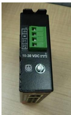
Wiring connection example. Pinout is NOT typical for all models.
