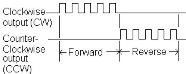
Mode 30 also allows several types of waveforms to be sent to the outputs. Let's go over the available options:
