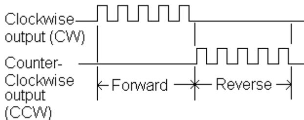
Mode 30 also allows several types of waveforms to be sent to the outputs. Let's go over the available options:
