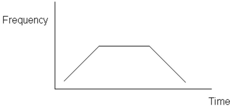
The 06 also includes a registration profile as part of the trapezoidal profile. The major difference is that the registration profile will continue to run at the target frequency until a separate pulse input indicates the profile should stop. The profile then decelerates and stops at a particular number of pulses **BEYOND** the point where the registration input occurred.
