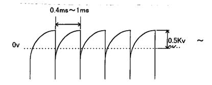
Wave height: Sweep between 0.5KV to 2KV manually.
