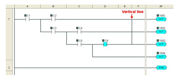
**Problem 3:** Coil and Box instructions may not work correctly when the For instruction is used in a rung with branches.
